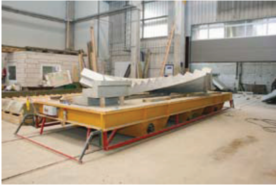
Fig. 2 The floor truck supplied by WMW in the production building.
